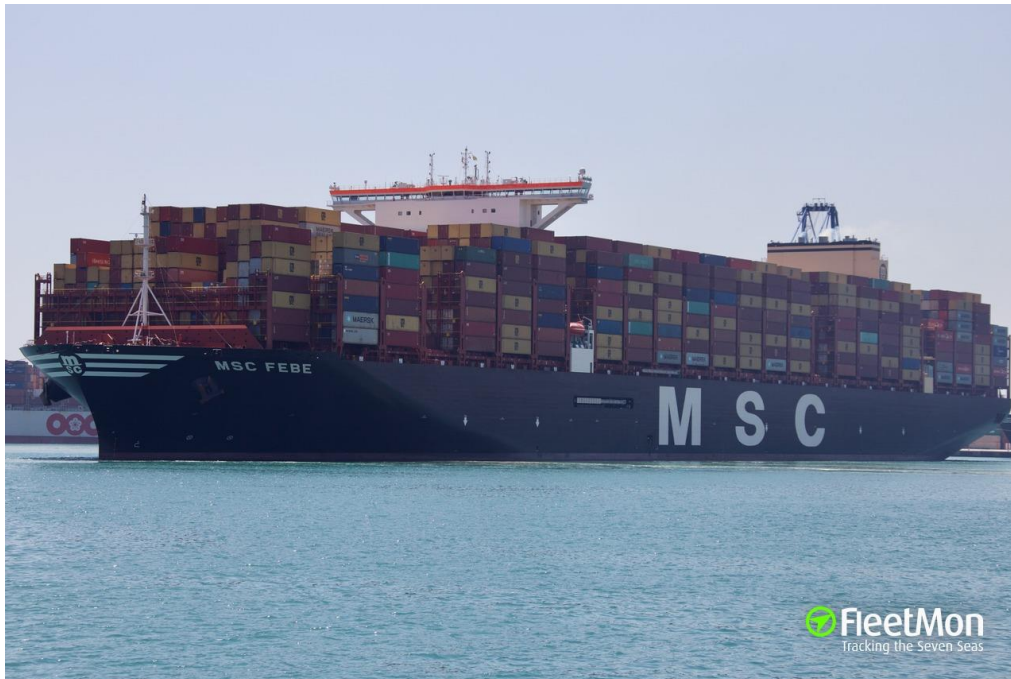
Scrubber equipped MSC Febe , built in 2019 is 399,9 mtr long and carries 23,756 TEU (twenty foot equivalent containers)
