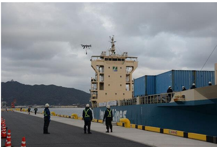
Drone with heaving line
